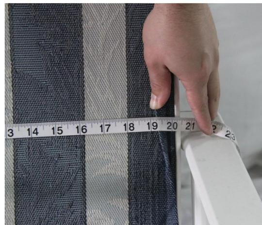
When measuring the frame for width, two measurements should be taken. Chair Care Patio has found it is best to measure in areas where the bolts and spreader bars are attached. For instance on a chair frame, measure the back of the chair near where the bolts attach and at the seat of the chair where the bolts attach near the knees.
