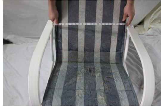
In most cases the fabric will be hiding the slot along the chair rail. Simply fold the fabric back to reveal the slot in the chair rail used for measuring. You will have to fold the fabric back on both sides so it may be useful to have an extra set of hands for this step.
